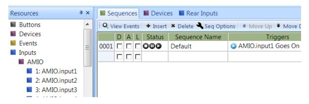
Drag the inputs into the "Sequences" view to easily create triggers. (Shown above)
