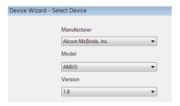
Select the "Make", "Model" and "Version" for the AMI/O as shown above. The version number may increment as slight changes are released.
