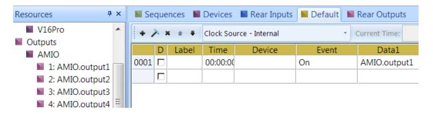
Similarly, outputs can be dragged into the "Events" view to turn on and off an output.
