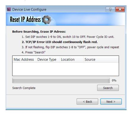
Before the AMI/O will appear, the IP address must be erased and the "ERROR" led on the front of the AMI/O must be blinking red.
