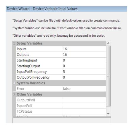
Enter the desired number of inputs and outputs for the show controller to control using the "Inputs" and "Outputs" fields.
