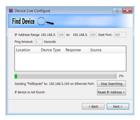
Each IP address in the range will be "pinged" by the show controller and will try to establish a response to the Modbus TCP command of "Poll Inputs".
