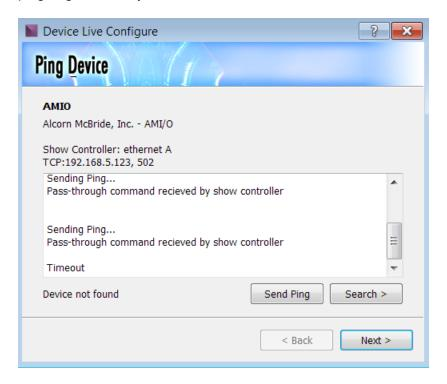
If the "ping" log window shows "reply received", no further configuration is nessessary. Your AMI/O is ready to use with the show controller.
