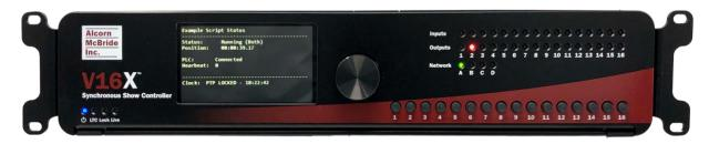
In this system, the V16X is responsible for commanding the Binloop to play different clips. This can happen as a result of touch panel buttons, IO (motion sensors, physical buttons, etc.), or clock-based scheduling. The V16X is also required to provides touch panel functionality using our ShowTouch panels or Apps. kind of flexibility and much more.
