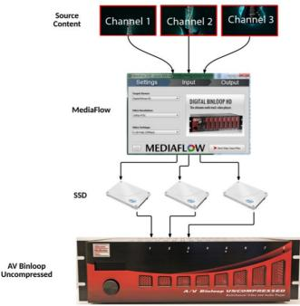
The quickest and easiest way to load content to the SSD drives is by interfacing to them directly from a computer using a SATA adapter. A USB 3.0 SATA adapter is included with every AV Binloop Uncompressed for this purpose.
