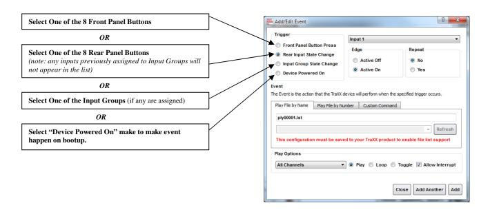
The best way to cause the 8TraXX/E to play something on startup is to select the *Device Powered On Trigger Type*.
