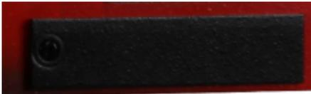
Secured with a screw, the metal cover can be removed to reveal the compact flash card. LightCue ships with a 4GB flash card. All data with the exception of the IP address is stored on this card.
