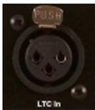
Female 3-Pin XLR. Transformer coupled 600 ohm Balanced -10 dbu to +4 dbu
