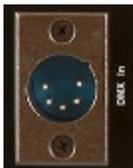
Female 5-Pin XLR. Used for record and feedthrough.
