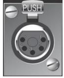
This is a 5-Pin female XLR connector used to connect a microphone and push-to-talk(PTT) switch. The ProTraXX can route the microphone input to any channels or group of channels. See the section on "Microphone Paging" for additional details.
