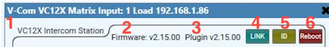
7. **Status Bar:** A graphic representation of an active VC12X hardware. (Red: Disconnected. Green: Connected) New with Plugin v2.15.00, this bar will also indicate if you have a firmware/plugin mismatch.
