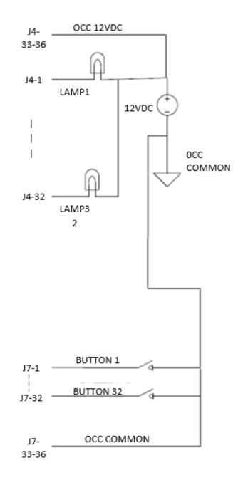
NOTE: FOR INSTALLATIONS THAT DO NOT HAVE AN EXTERNAL OCC POWER SUPPLY INSTALL JP5 AND JP6 JUMPERS IN 2-3 POSITION TO USE INTERNAL VPAGE32 POWER. OTHERWISE INSTALL IN 1-2 POSITION.
