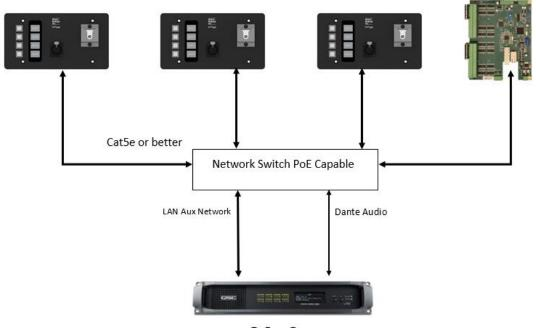
VP32K and VP4X Stations via Ethernet cables and Dante audio
