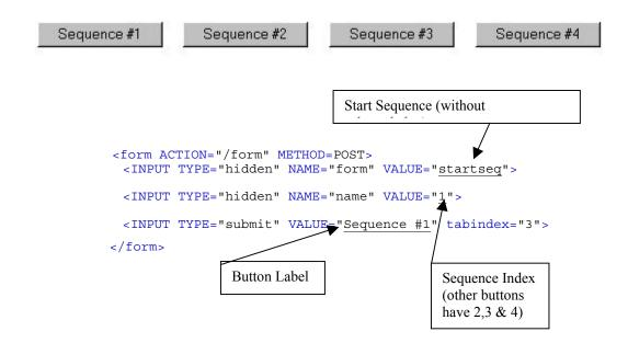
Notice that no acknowledgement from the show controller is expected in this example. The unit does not automatically send an acknowledgement when the Programmer port is used. This can program this into your script however, and use the next example if you need feedback from the controller.
