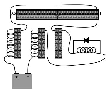
Figure 4 – A relay or solenoid is a common example of an inductive load and must have a 1N4000-Series snubber diode placed across it. Be sure to observe proper polarity (anode to negative side).
