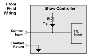
Figure 1 – Contact Closure Schematic.
