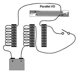
Figure 3 – Sample connection for a Voltage Input to Input9 of the Parallel I/O connector. The terminal blocks are used for power bussing and modularization of the input signals.
