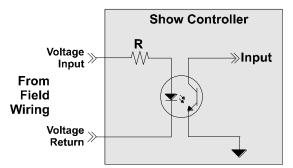
Figure 2 – Voltage Input Schematic.
