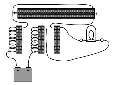
Figure 3 – An indicator lamp is a common example of a non-inductive load.
