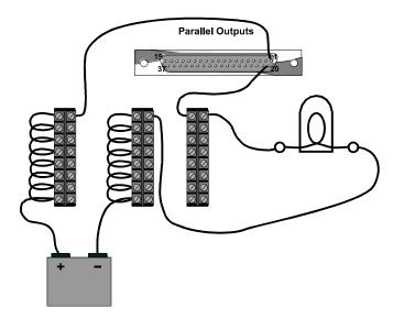
Figure 6 – An indicator lamp is a common example of a non-inductive load.
