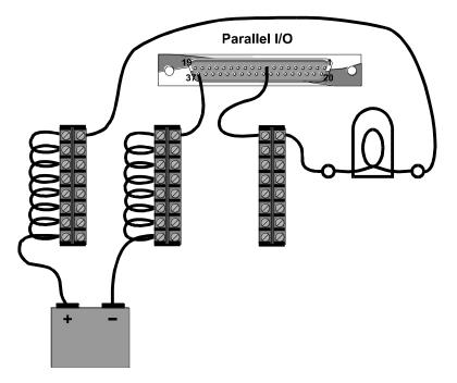
Figure 5 – An indicator lamp is a common example of a non-inductive load. This one is connected to the "Running" output.
