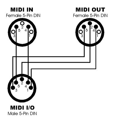
Figure 1 – IO64 MIDI Input/Output Cable.
