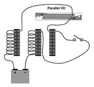
Figure 3 – Sample connection for a Voltage Input to the "Start" input of the Parallel I/O connector. The terminal blocks are used for power bussing and modularization of the input signals.
