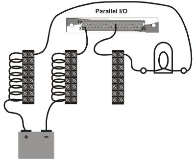
Figure 5 – An indicator lamp is a common example of a non-inductive load.
