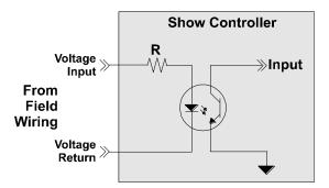
Figure 2 – Voltage Input Schematic.
