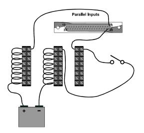
Figure 4 – Sample connection for a Voltage Input to Input1 of the Parallel Inputs connector. The terminal blocks are used for power bussing and modularization of the input signals.
