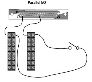
Figure 4 – Sample connection for a Contact Closure Input to Input9 of the Parallel I/O connector.
