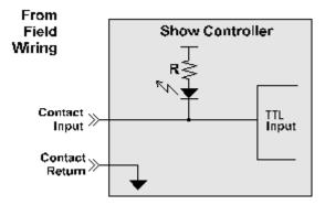
Figure 1 – Contact Closure Schematic.
