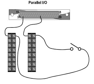
*Figure 4 – Sample connection for a Contact Closure Input to the "Start" input of the Parallel I/O connector*
