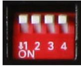
Four small DIP switches on the side of the unit are used to configure various hardware related settings.
