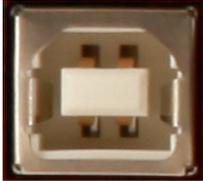
TourTraXX includes a female type-B USB connector on its front panel. This port can be used to control TourTraXX, using its standard command set, as a USB serial device. While many operating systems will detect and install the driver automatically, some operating systems such as Windows 7 64-bit will need the user to supply the appropriate driver. This driver is available from our website, at <http://www.alcorn.com>.
